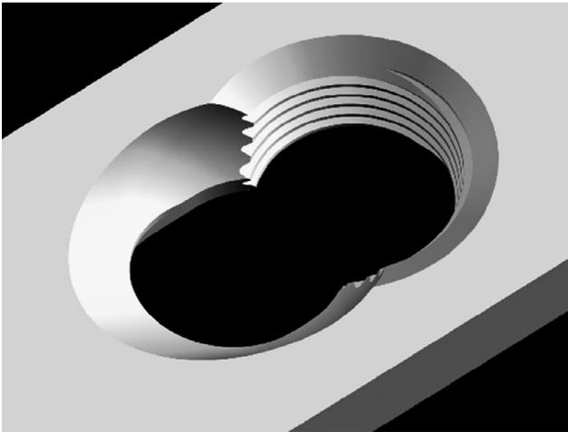
Figure 1. Combination hole as principle of the LCP gives surgeons the opportunity to combine principles of internal fixation and dynamic compression, depending on the fracture site.
