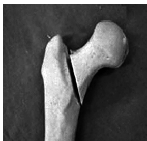
Fig. 1. Standard Pauwels type 3 basicervical femoral neck fracture with an angle of 70° osteotomy in synthetic bone model.
